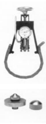
Used for large cylinders it fits onto a standard test head and wraps around specimens that are too big for regular tester. High strength chrome/molybdenum steel arms hold the chain to the test head and allow it to stay rigid while the chain takes the full thrust of the load. Supplied with 4' chain.
